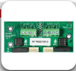
Interface for cable connection between a G-ONE, Gekko, or Octo+ panel and a Chameleon Display repeater
