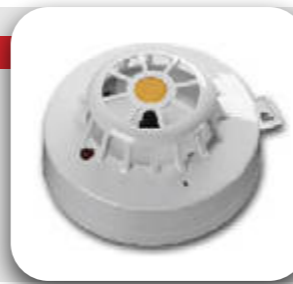
Apollo addressable heat detector. • Monitors ambient temperature with a thermostat, triggering an alarm at 55 °C. • Ideal for areas with impurities or smoke under normal conditions. • Working temperature: -20°C to +70°C. • Unaffected by wind and atmospheric pressure. • XP95 Apollo protocol.
