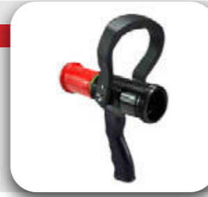
Plastic 2" branch pipe with adjustable water beam. • Certified. • Technical specifications: • Operating pressure 4 -15 bar, flow 500lt/min at 7 bar. • With 2" coupling (included). • K-factor: K-217 (spray) / K-133 (direct shot).
