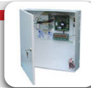
External power supply ORION BCM LSC. • It connects to Globalfire addressable systems on the loop and occupies 2 addresses on the loop. • It has a separate output for a conventional siren, which can participate in the system's cause-effect scenarios through scenarios. • Ideal also for door electromagnets. • Requires 2 batteries 12V - 7Ah, which are not included in the cost. • Certified according to EN54-4.
