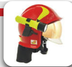
Firefighting helmet. Manufactured and certified according to EN443:2008, type B with C sticker for chemical resistance. Adjustable circumference range: 53–62cm. Weight: 1.650gr. Supplied with two visors, certified according to EN14458:2004. Equipped with detachable fire-resistant neck protector, adjustable chin strap made of flame-retardant material, and bracket for attaching a flashlight (UK 4AA type). Compatible with self-contained breathing apparatus (SCBA) mask visors.
