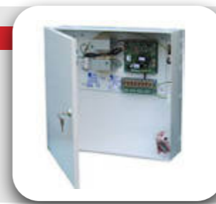
Power supply unit 24V-4Ah. (Required 12V-4.5Ah batteries not included) • Batteries voltage monitoring. • Built-in output for conventional sounder beacon. • Two relays included (Fault & Fire). • EN54 certified.
