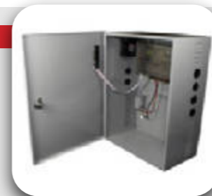
Power supply unit 24V-10Ah. (Required 12V-7Ah batteries not included) • Power supply with battery charging mode, housed in a metallic enclosure. • Provides protection against battery overcharging and undercharging. • Supply voltage: 220V AC. • Size: 395x285x165mm • Weight: 6kg. • Color: grey.
