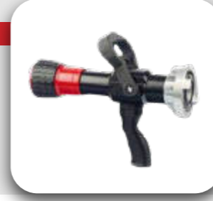
Aluminium 2" branch pipe with adjustable water beam. • Certified. • Technical specifications: • Operating pressure 4 -15 bar, flow 500lt/min at 7 bar. • With 2" coupling (included). • K-factor: K-217 (spray) / K-133 (direct shot).
