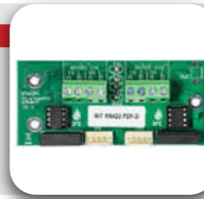
Interface for remote network monitoring and control of the fire detection system via the Global Fire platform. (for G-ONE, Gekko & Octo+ panels)
